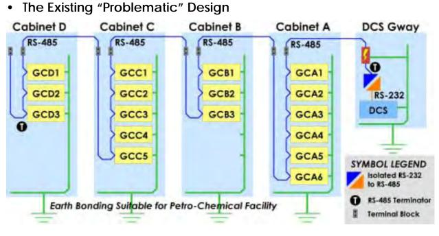
The original design has all of the devices on a single RS-485 network. Only the DCS gateway device is well designed with appropriate surge protection. The original design has no surge protection in the field cabinets. Below is a quick analysis of the "Robustness Factors" (N/C means we don't plan to change or No-Change). We have 18 devices on one 600m RS-485 bus. Every wire has about 72 points for mechanical failure – meaning the 4-wire RS-485 network has almost 300 screws to come loose.
