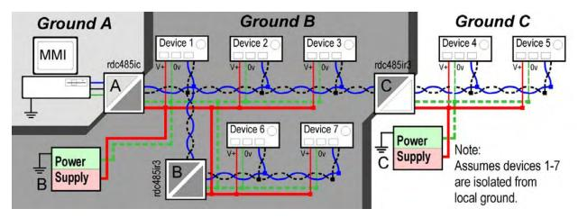
This application example shows the use of 2 units of rdc485ir3 and 1 unit of rdc485ic to expand the design of a 4-wire network with RS-485 and a 24vdc power bus. The RS-485 is shown as the twisted wire pair. The 24vdc power bus is shown as the heavier wire pair. One computer and two power supplies are used. Since all the field devices 1-7 are isolated from the field ground, the isolation inherent within the rdc485ic and
