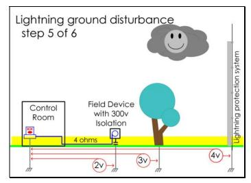
vaguely that the law of Conservation of Energy says it cannot disappear. It will eventually be attracted to some remote location to due to the creation of lightning-causing potentials. In fact, the ground charges are to lightning much like water is to rain.
