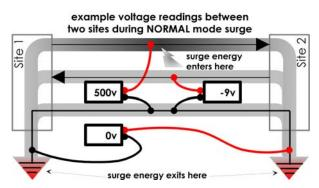
one pin having a high voltage. In this example, a 500v noise spike was induced on one wire and travels outwards towards both remote grounds.
