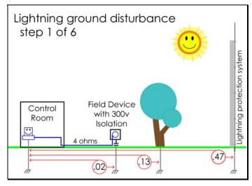
could potentially have about 5mA of ground current flowing from the field device to the computer through the RS-232 port. This would be known as a "ground loop" and is why most 4-20mA loop devices (like pressure or temperature transmitters) are carefully isolated. It must be stressed that the actual values during ground potential disturbances are in a constant state of flux. This is just a simple, non-destructive example.
