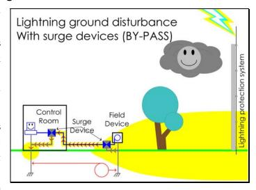
over-voltage conditions exist, the surge device must rapidly "break-down" and appear as a low-impedance path to ground. They effectively short the wire to ground to discharge the surge (or allow the ground surge to enter!) The first concern is of course the speed of this change, and the second is that if your device already offers a low-impedance path to ground, then a surge device cannot provide a lower one and will not work.
