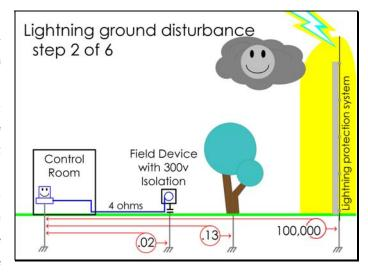
exact number is not important, other than it's more than you want. The background shading in this drawing and the following ones represents visually the voltage potential movement.
