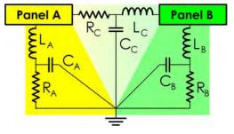
Another way to view the problem is shown at left. With 2 panels (whether 1 or 2 vendors) you have subtly different electrical characteristics on the ground/earth wire. Here we have inductance (L<sub>A</sub>), resistance (R<sub>A</sub>), and capacitance (C<sub>A</sub>) from panel A to site ground. We also have  $L_B/R_B/C_B$  for panel B and  $L_C/R_C/C_C$  on the data communication line between the 2 panels. So the question is - "during a surge or ground fault
