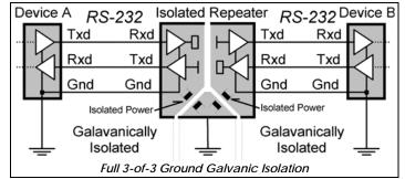
physical layout of your system. 3-port isolation allows a natural physical arrangement where a computer (device A) is located in the control room, the isolated repeater is located in marshaling panels, and the
